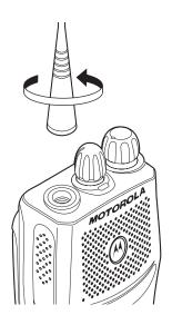
Turn the antenna counter-clockwise to remove it.
