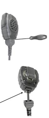
4. Insert the small flathead screwdriver under the locking tab of the RJ45 connector and push the tab up.  $_{\sim\!\!\!\sim\!\!\!\sim}$
