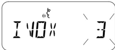
If VOX is enabled (with accessory connected to the radio) when you press the (Menu) button, the radio displays the following:
