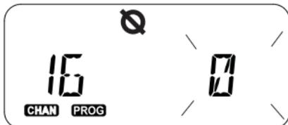
The current scramble value blinks. You can select the desired scramble value (0,1,2 or 3) by pressing the and buttons. Long press the PTT button to exit and save, or short press the PTT button to move to the next programming feature without saving.
