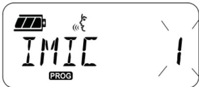
The radio display blinks the current Microphone Gain Level setting. You can select the desired Microphone Gain Level (1 = low gain, 2 = medium gain or 3 = high gain) by pressing the Programmable Button A and Programmable Button B buttons.
