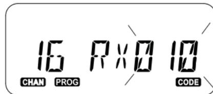
To program the desired code, use the and buttons until you get the CTCSS/DPL code value you want to set up. Long press the PTT button to exit and save, or short press the PTT button to move to the next programming feature without saving.
