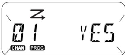
Both the channel number and current scan setting (YES = Enable or NO = Disable) blinks on the display, indicating you can choose your setting. To set the channel number, rotate the Channel Selector Knob until you reach the desired channel number.
