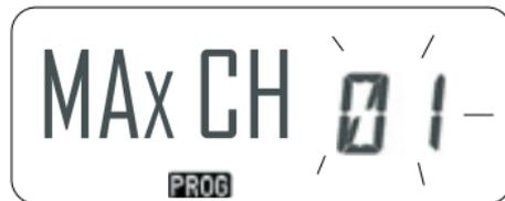
The radio display blinks the current maximum number of channels programmed. Use the Programmable Button A and Programmable Button B buttons until you get the desired maximum number of channels. Long press the PTT button to exit and save, or short
