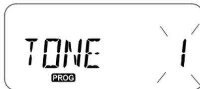
The radio display blinks the current call tone setting. You can select the desired call tone value (0,1,2 or 3) by pressing the Programmable Button A and Programmable Button B buttons. Each time you select a different value, your radio sounds the selected call tone (except for value '0'). Once you have selected the desired call tone, long press the PTT button to exit and save, or short press the PTT button to move to the next programming feature without saving.
