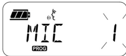
The radio blinks the current Microphone Accessory Gain Level setting. You can select the desired Microphone Accessory Gain Level (1 = low gain, 2 = medium gain or 3 = high gain) by pressing the Programmable Button A and Programmable Button B buttons.
