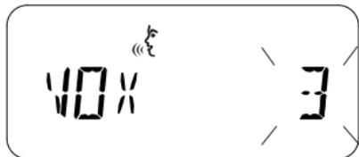
To change the sensitivity level, use the Programmable Button A and Programmable Button B buttons:
